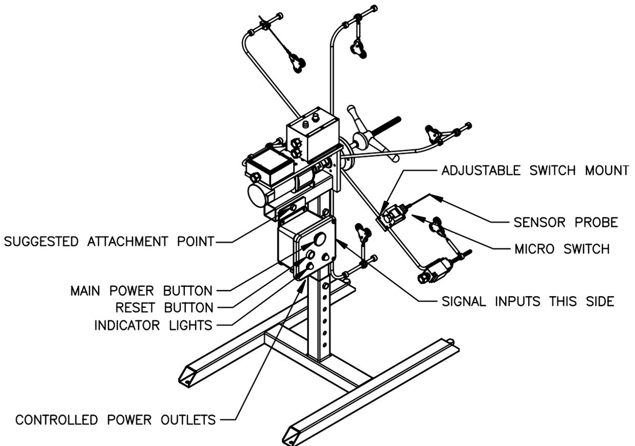
This system is designed to provide an automatic shutdown of any equipment attached to the controlled outlets. This system also requires a “manual reset” to restore power to any equipment attached to the controlled outlets.
