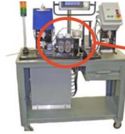
Prior to stacking, a crown shape is rolled into the strip using the feed rolls
