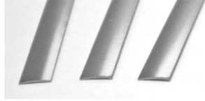
Prior to stacking, a crown shape is rolled into the strip using the feed rolls
