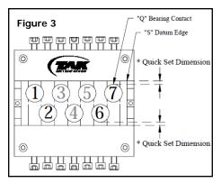
ed settings for specific wire diameters are indicated. We start with a "QS", or Quick Set dimension, which is the dimension to set the leadin bearings at the point that they just make contact with the wire. From there, setting dimensions for percentages of wire break on the remainder of the bearings are listed. Click on the link at the bottom of this page in the blue box which will bring you to the standard **TAK PWS**
