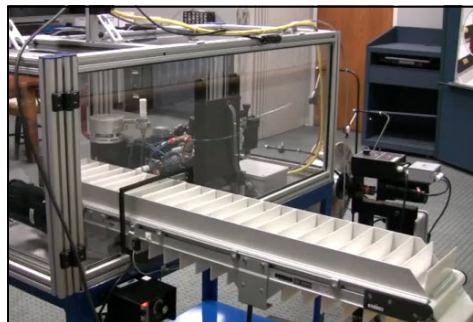
A standard conveyor with a lugged belt is used to provide compartments for segregating the batches
