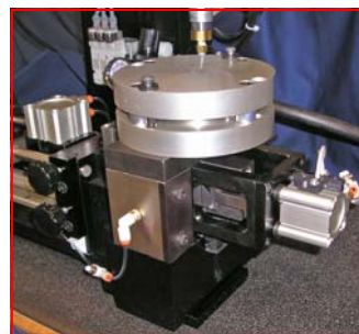
Special Cutter Head Provides Motions to Support OD and ID on Both Ends of Cut Surfaces to Minimize Distortion and Provide Burr-Free Shear Cut
