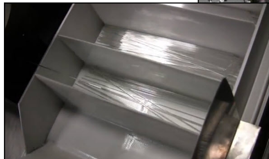
Wire feeds into position above the conveyor compartment. After the shear cut, the next feed cycle ejects the cut wire and it drops into the conveyor compartment
