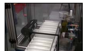
Sensors are used to locate the conveyor lugs after each advance
