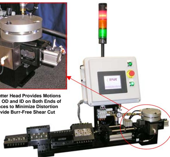
TAK #2 SFC Tube Shearing System
