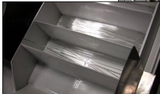
Wire feeds into position above the conveyor compartment. After the shear cut, the next feed cycle ejects the cut wire and it drops into the conveyor compartment
