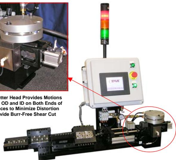
TAK #2 SFC Tube Shearing System
