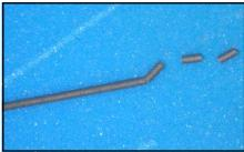
Voids and cracks in the extruded material proved to make it too delicate to withstand enough conventional feed roll grip pressure to advance it at the required rate.
