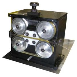
The Dual Belt Tractor Feed utilizes 2 opposing cog belts to spread out the gripping force over a large area. Rubber belts proved to provide enough traction without distortion or breakage of the brittle material.
