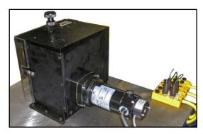
Running as a slave to a specialized press, a single axis servo drive and motor read a signal from the pressmounted encoder to deliver the required amount and speed of the material to be fed.
