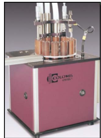
The Colombi Orbit inspects each spring for load value and delivers only good springs
