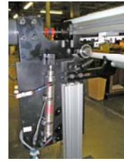
Conveyor-Dump Tray Actuation Mechanism
