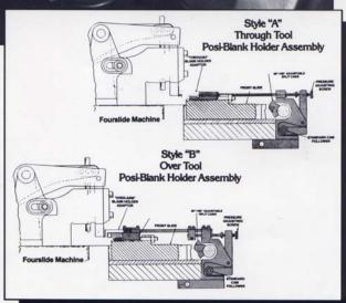
The Posi-Blank Holder Style "B" is specifically designed for easy adaptation to your machine with no modification. It may also be used on present tooling with very little alteration.
