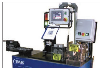
Photos (top to bottom): Automated Abrasive Wheel Cutting Station ( Guards removed for clarity ); Cut Ends on Steel Jacketed Coaxial Cable; Servo Feed and Cutoff System for Jacketed Coaxial Cable Cut to Various Lengths
