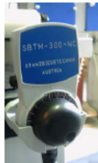
Operating Terminal with Jog-Buttons and Electronic Hand-Wheel.
